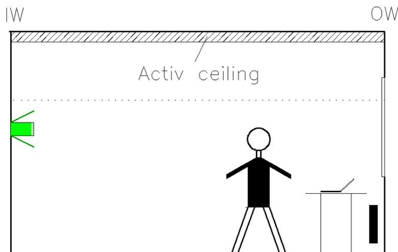
Figure 2-4 Possible position of the infra-red camera in the room with heated/cooled ceiling
