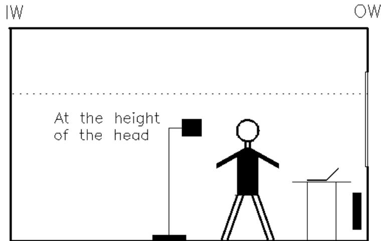
Figure 2-8 Pollutant concentration measurement in the zone of person's stay
