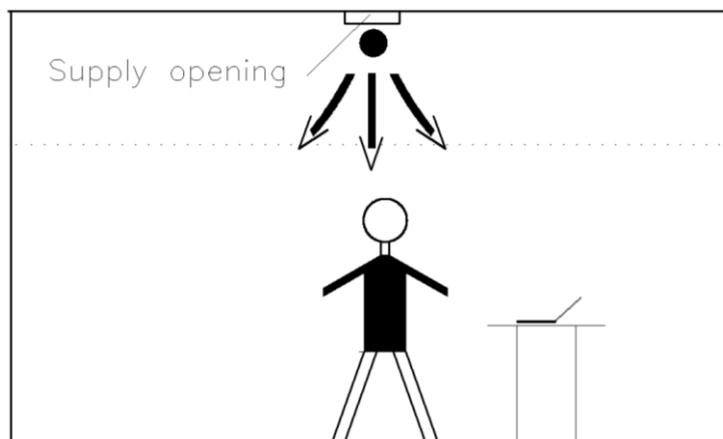
Figure 2-6 Air velocity measurement with unidirectional/bidirectional anemometers in front of the supply opening
