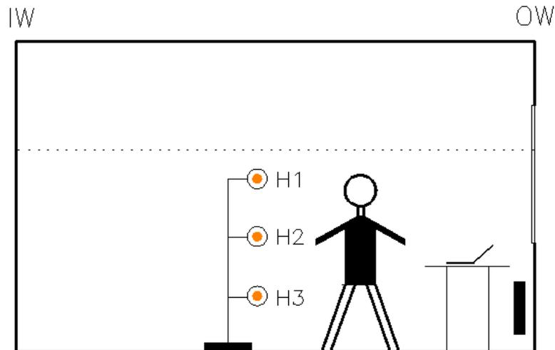
Figure 2-1 Air temperature measurement in the zone of person's stay
