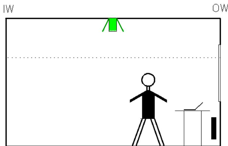
Figure 2-3 Possible position of infra-red camera
