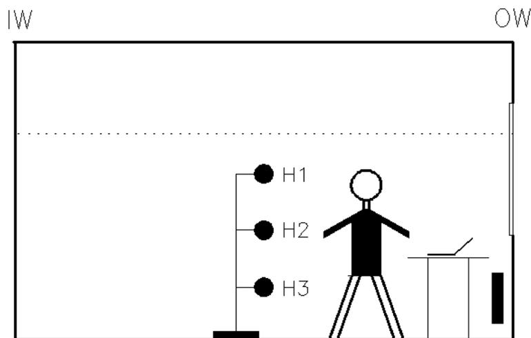
Figure 2-5 Air velocity measurement with omnidirectional anemometers in the residential zone
