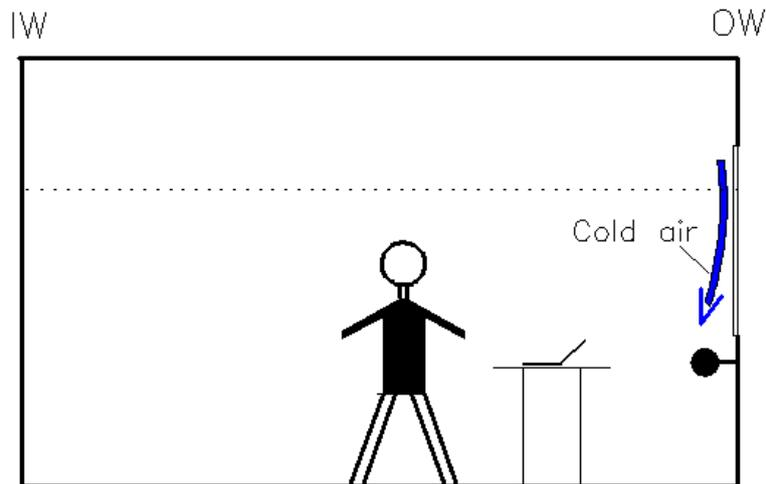
Figure 2-7 Air velocity measurement with unidirectional/bidirectional anemometers under the window
